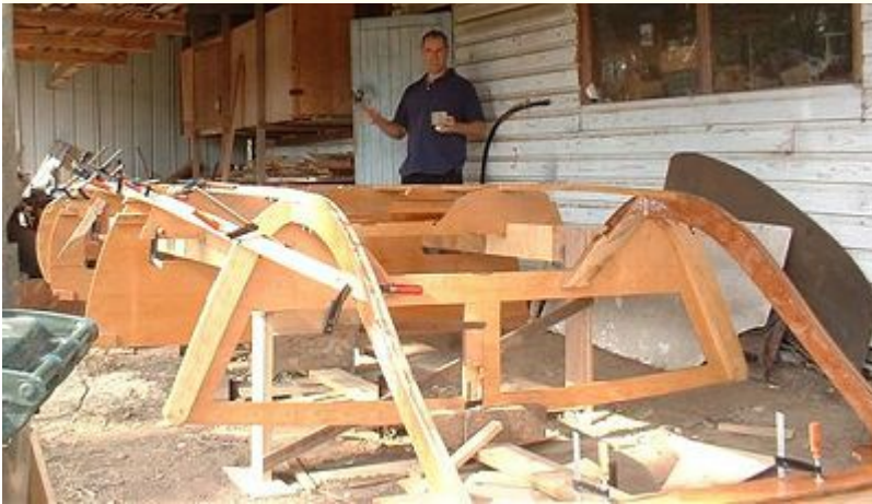
First chine log installed as a mate brushes on some more epoxy.
