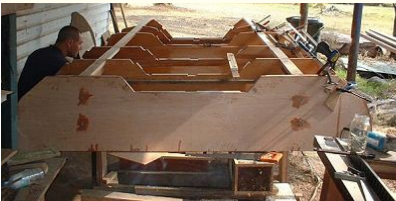
Transom in place and some assistance being given from a mate.
