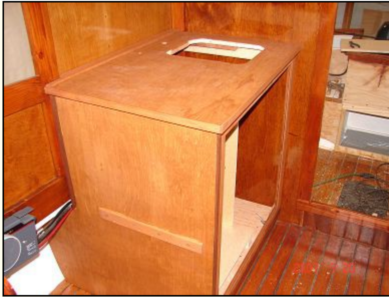
The galley cabinet taking shape. There will be a small twelve-volt fridge in there.
