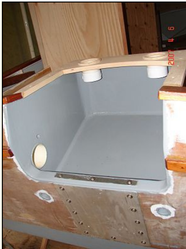
Here is a picture of the motor well. I installed aluminum plates so the motor does not hang directly on the fiberglass. The tube on the left hand side is for the steering cable/rod.
