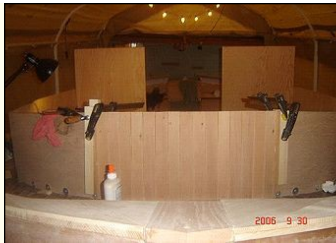
This is the front of the trunk cabin. I'm gluing on DF strips. They're 1\frac{3}{4} inches wide and \frac{3}{16} inches thick. They will be on the entire outside of the cabin.
