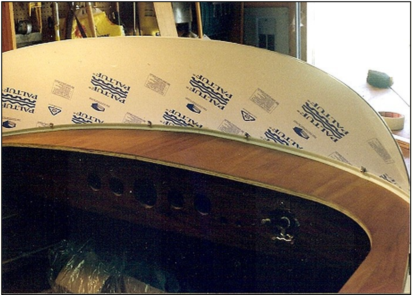
Windshield with protective film still attached. Hold downs and deck channel are in place.
