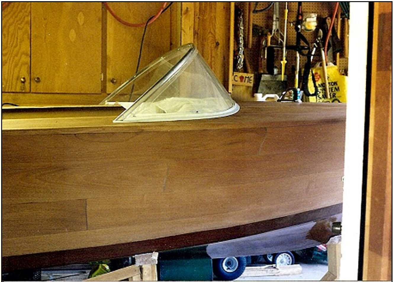
Side view of finished windshield with deck channel ends trimmed. White protective film has fallen from the Lexan but clear film is still trying to hold on. I left the protective films on as long as possible.
