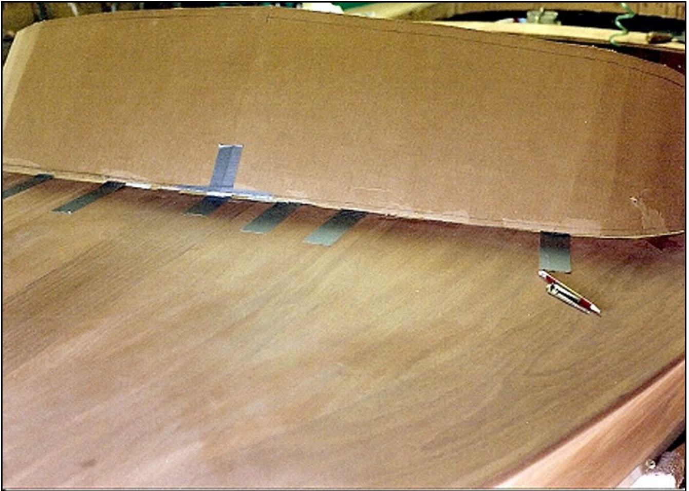
Cardboard template taped in-place. I used a scribe to mark a fair line along the deck edge of the windshield template.
