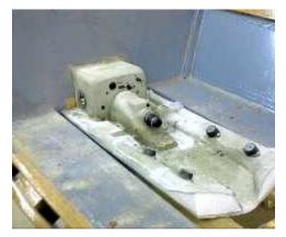
The Seadoo hull cut to size. Notice the composite hull contruction. I used 6" lag bolts to tie the two hulls together and self-rising foam to fill the gap between the Seadoo and Jetfish shoe. Once fiberglassed the afte deck will be level.
