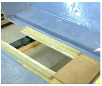
Poor old Jetfish has her bottom cut out yet again! I'm thinking of renaming her "Patches". You can see the treated boards cut on an angle to match the Seadoo hull.
