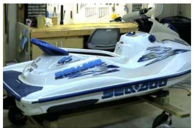
Here's the "donor" craft ready to undergo radical surgery. Begin by removing all the stuff fastened to the top half of the hull.
