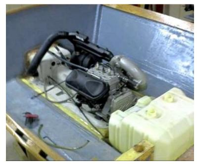
After adding three new layers of 9oz. glass to the bottom, two fresh coats of electric blue epoxy paint, and tearing down the engine for inspection, it was time for a trial fit. Because I really wanted to use the Seadoo fuel tank, I cut the center out of the bulkhead. Next step is inventing some steering and (hopefully) breeding the GTX reverse gate to the GS pump. Note the Seadoo hull fit Jetfish's shoe like a glove.
