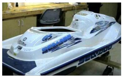
Once everything has been removed (including wires and fuel lines positioned along the sides) its time to saw all the way around the hull seams. I cut just inside the blue rubber bumper.
