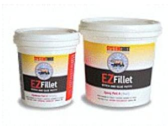
EZ-Fillet is a wood flour-filled two-part putty specifically designed for stitch-and-glue wooden boat construction. Its ketchup-like, self-leveling consistency allows it to be measured by volume or weight. The resin (part A) is brick red in color while the hardener (part B) is a deep, dark green. A rich brown wood tone results when the two parts are combined indicating complete mixing.
