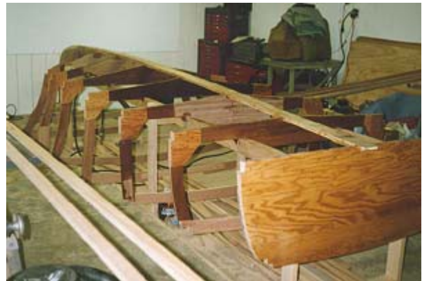
Fig. 2 - Hull frame and backbone member contours are taken from FULL SIZE PATTERNS , built and set in place on the jig. Frames have been pre-coated with epoxy resin as part of our recommended EPOXY ENCAPSULATION system that locks out moisture to stabilize the wood, prevent rot, and eliminate maintenance. The same resin can also be used for gluing parts together.
