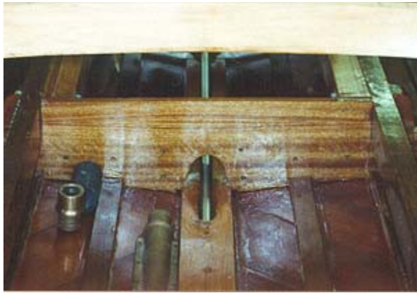
Fig. 9 - Motor has been installed along with the propeller shaft visible here. Hull is ready to be decked over now.
