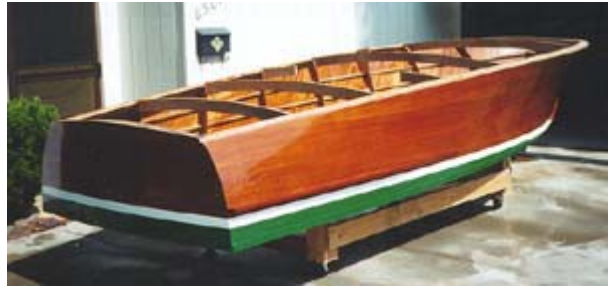
Fig. 6 - Completed hull has been removed from jig and righted for the balance of construction. John rigged up a dolly here, but you could also use the boat's trailer at this point. We have BOAT TRAILER PLANS that you can use to build your own.
