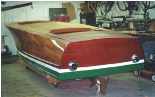
Fig. 11 - Hull with plywood subdeck in place is ready for final deck. Note that the transom is not just a slab of flat plywood - plans include easy methods for making the authentic curved type without grief or hard work.
