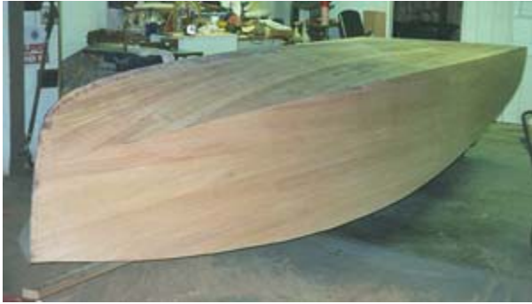
Fig. 5 - Final planking layer is applied lengthwise to emulate traditional planking of the past. John did the bottom this way also, but double diagonal format here is optional as well. Hull is now ready for fiberglass cloth & epoxy sheathing as provided in our FIBERGLASS COVERING KITS .
