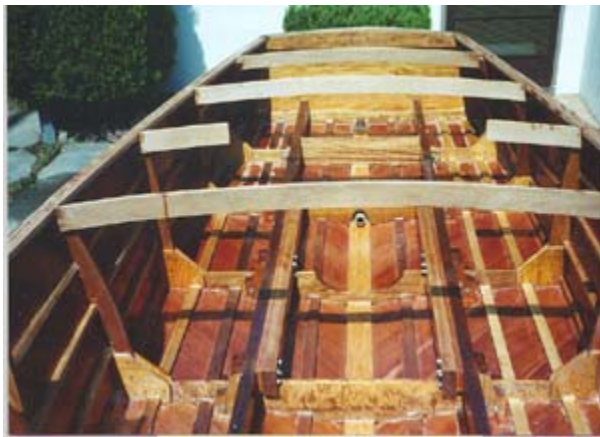
Fig. 7 - Hull is ready for the motor installation. Note husky stringers and adjoining motor beds bolted along the inside of these. Hull was bored for shaft while upside down. Note how all surfaces are coated with moisture-inhibiting epoxy.
