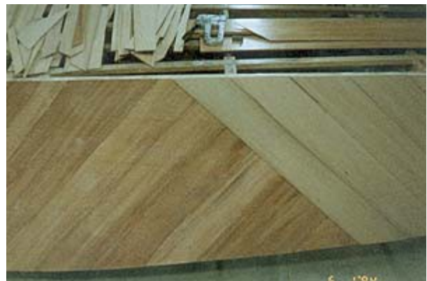
Fig. 2 - Hull frame and backbone member contours are taken from FULL SIZE PATTERNS , built and set in place on the jig. Frames have been pre-coated with epoxy resin as part of our recommended EPOXY ENCAPSULATION system that locks out moisture to stabilize the wood, prevent rot, and eliminate maintenance. The same resin can also be used for gluing parts together.
