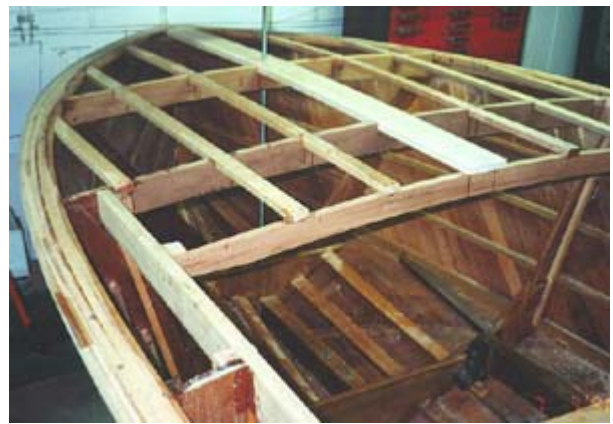
Fig. 10 - Decking is supported by a strong framework. The vertical rod is for an optional lifting eye; another will be installed aft.
