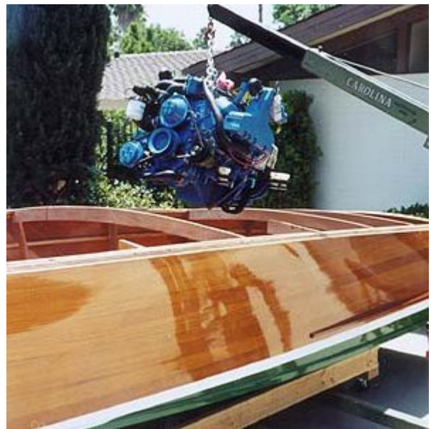
Fig. 8 - John picked a new CRUSADER V-6 for his boat, a compact, lightweight motor with plenty of power. You could also convert your own automotive motor to marine use if you like.
