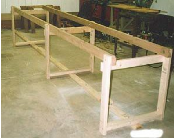
Fig. 1 - Hull construction is done upside down over a simple building form or "jig". The top lengthwise members are the motor stringers that stay in the boat and are notched to receive the frames of the boat.
