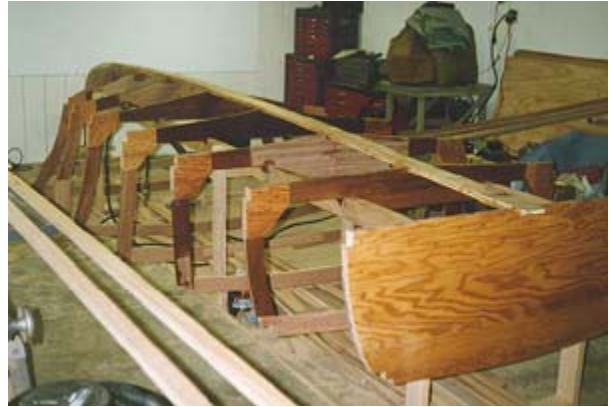
Fig. 2 - Hull frame and backbone member contours are taken from FULL SIZE PATTERNS , built and set in place on the jig. Frames have been pre-coated with epoxy resin as part of our recommended EPOXY ENCAPSULATION system that locks out moisture to stabilize the wood, prevent rot, and eliminate maintenance. The same resin can also be used for gluing parts together.
