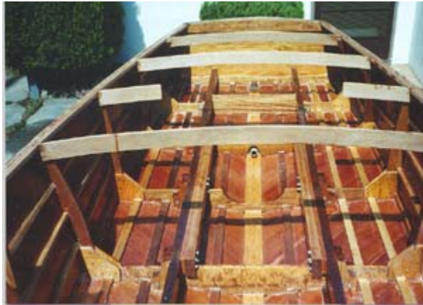
Fig. 7 - Hull is ready for the motor installation. Note husky stringers and adjoining motor beds bolted along the inside of these. Hull was bored for shaft while upside down. Note how all surfaces are coated with moisture-inhibiting epoxy.
