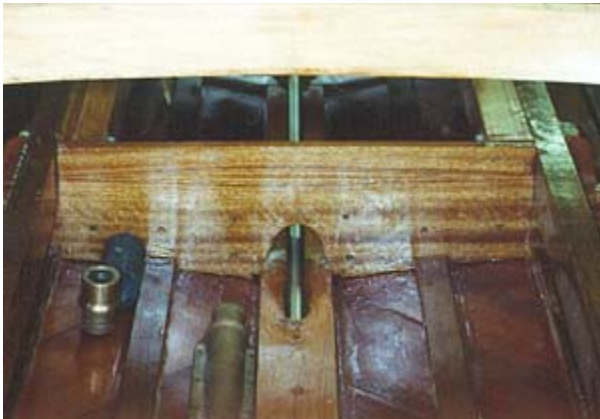
Fig. 7 - Hull is ready for the motor installation. Note husky stringers and adjoining motor beds bolted along the inside of these. Hull was bored for shaft while upside down. Note how all surfaces are coated with moisture-inhibiting epoxy.
