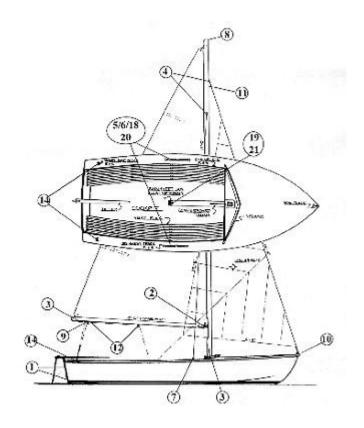
pass under. Bolt pintles to rudder with 10-24 round head machine screws. Fasten gudgeons to transom with 10-24 machine screws or #8 round head wood screws. The rudder stop (angle) will mount to transom centerline approx. 5/8" above top gudgeon. Use #6 RH screw, do not tighten all the way, it should easily pivot out of the way when the the rudder is installed. This piece is meant to keep the rudder from floating out.
