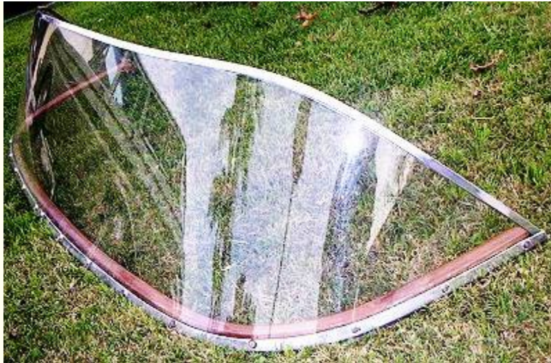
Photo #12. I built the windshield so it would come off easily. 5 wing nuts through the deck and 1 at each end through the covering boards.
