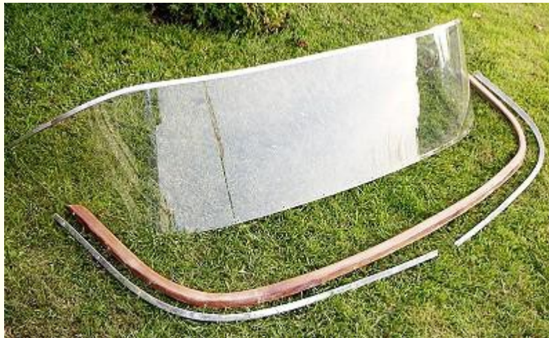
Photo #13. These are the parts that that make up the windshield. 1/8th inch Lexan/polycarbonate plastic. Aluminum channel for the top molding, 3/4" or 1" angle aluminum for the bottom molding and a wooden form/base mount to shape the bottom molding around.
