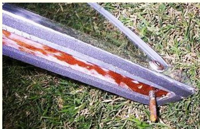
Photo #13. These are the parts that that make up the windshield. 1/8th inch Lexan/polycarbonate plastic. Aluminum channel for the top molding, 3/4" or 1" angle aluminum for the bottom molding and a wooden form/base mount to shape the bottom molding around.
