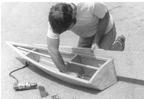
Fig. 19: The RUNNER SIDE PLANKING #11 is fitted oversize as shown. The only area that must be fitted carefully now is that portion forward of FRAME #3 which will butt to the RUNNER BOTTOM #12.
