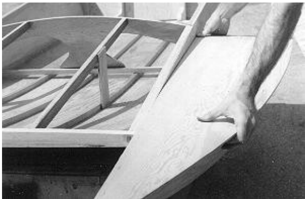
Fig. 31: The pre-fitted RUNNER DECKING #13 is fastened in place after coating the inside with paint or preservative. Overhanging extremities may be trimmed to fit after fastening in place.
