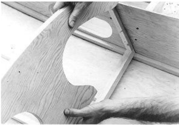
Fig. 24: The DASH BEAM #25 is fitted between the side planking, with the bottom portion bearing against the FORWARD BOTTOM FRAME #30 that has been angled 30^\circ .
