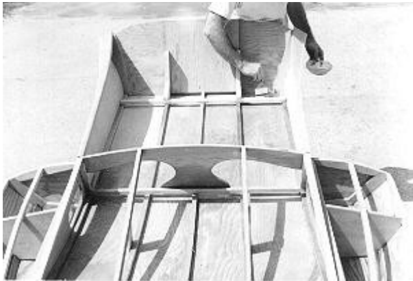
Fig. 30: The interior of the hull is coated with a preservative and then with a clear or paint finish prior to installation of decking.
