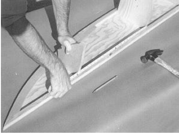
Fig. 1: The RUNNER SIDE #4 with the RUNNER KEEL #5, DECK CLEAT #6, and STEM#7 assembled to it. The frames are located on this assembly, spaced per the dimension sheet or as noted on the full size patterns.
