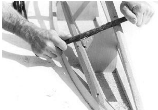
Fig. 10: One way to determine the amount of material to be removed is to file a notch to the required bevel on the longitudinal at the frames. In the forward area a wood rasp can be used to fair the RUNNER SHEER #8 and CHINE #10 simultaneously.
