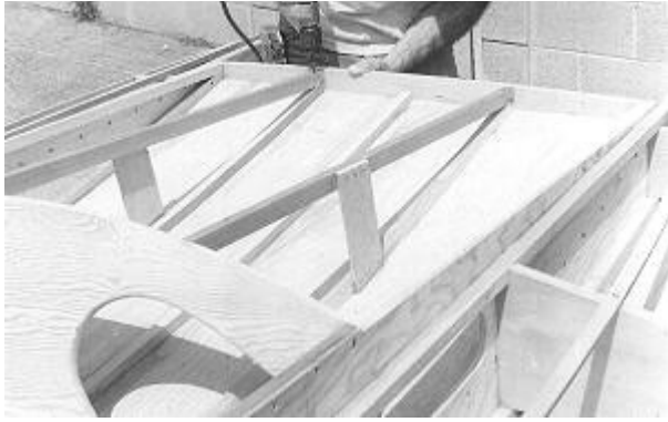
Fig. 26: The COWL BATTENS #26 are directly above the outermost two BOTTOM BATTENS #19. They butt to the DASH BEAM #25, bear on top of these bottom battens at the bow, and butt to the BOW PIECE #26.
