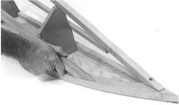
Fig. 4: The RUNNER CHINE #8 is beveled as shown to side to the STEM #7.
