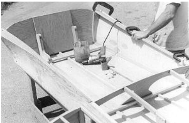
Fig. 28: The COAMINGS #29 are to extend beyond the transom for trimming to fit after fastening in place. The forward end must be angled to butt to the DASH BEAM #25. A considerable twist takes place in the COAMING #29 so use several clamps to hold the member in place while the fastenings are driven in.
