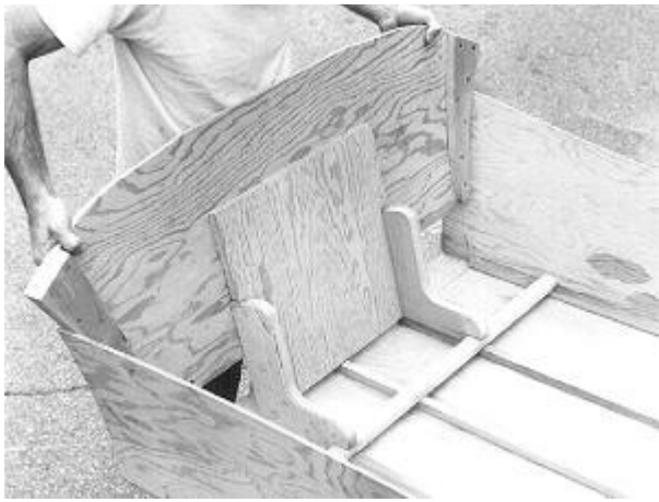
Fig. 27: The pre-assembled transom is slipped between the side planking to rest firmly on the bottom. Force securely against the inner motorboard. Liberal application of glue and solid bearing are important at this junction.
