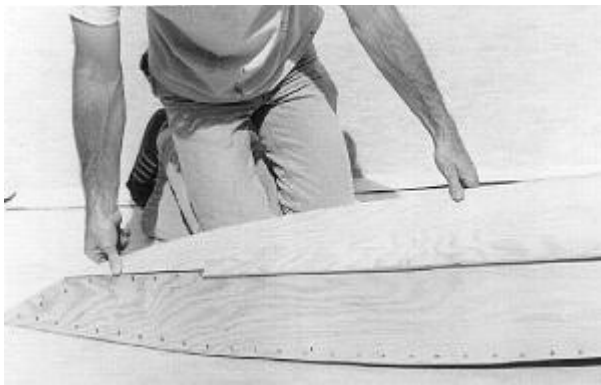
Fig. 18: The RUNNER SIDE PLANKING #11 is screwed in place after coating all mating areas with glue.
