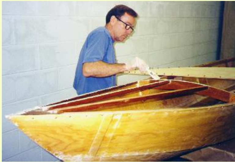
Applying thickened Poxy-Shield prior to installing the foredeck.
