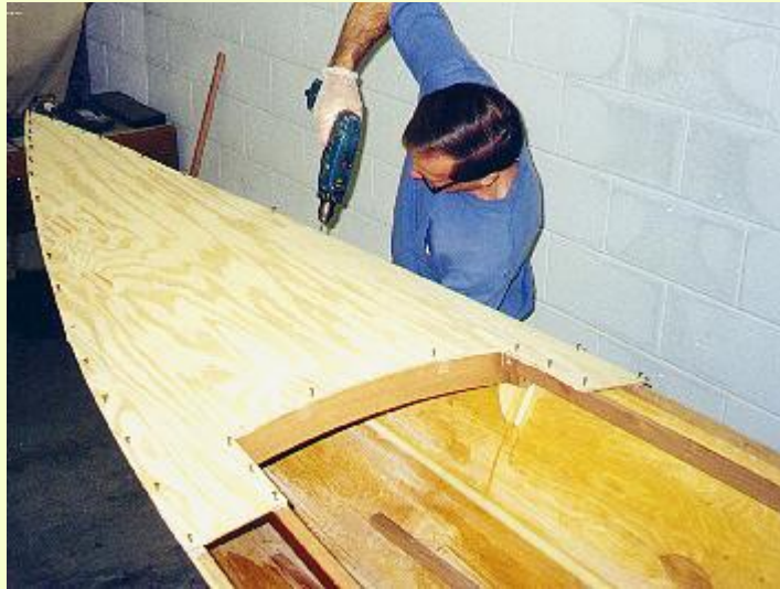
Installing the foredeck.
