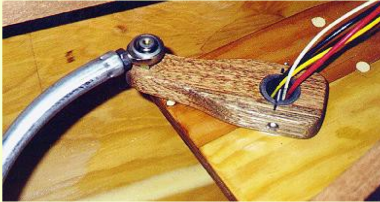
Control rod connection at the tiller.
