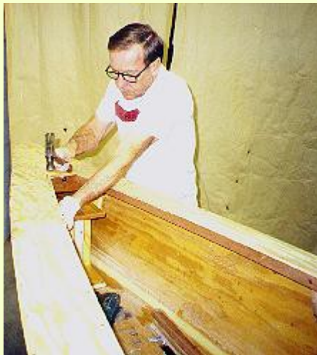
Installing the sidedecks.
