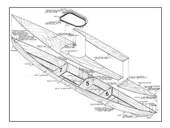
**Exploded construction drawing**
