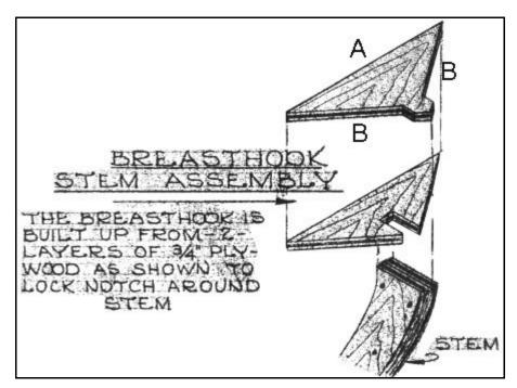
The Squirt breasthook is typical of most designs. The width of the notch in the lower half and the width of the piece the protrudes from the upper half should match the width of the stem. The protrusion on the front of the upper half should extend beyond the stem, far enough so that it can be faired to continue the stem contour.
