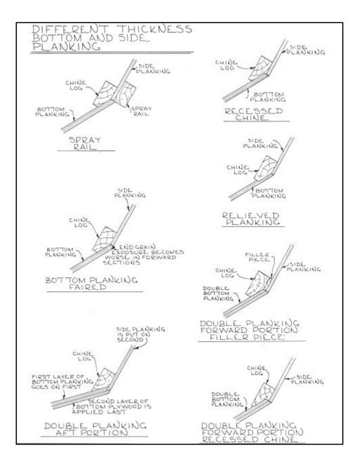
**Plate 19-E** - Methods for handling thickness variations between side and bottom planking at junctions over chine log. (*From BOATBUILDING WITH PLYWOOD*)
