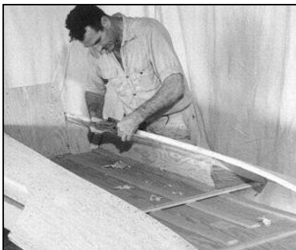
Fig. 10: Fitting of the decking need not be closely done as it can be trimmed after fastening in place. The area along the carling that will mate to the coaming should be carefully trimmed to provide a vertical surface for attaching the coaming.
