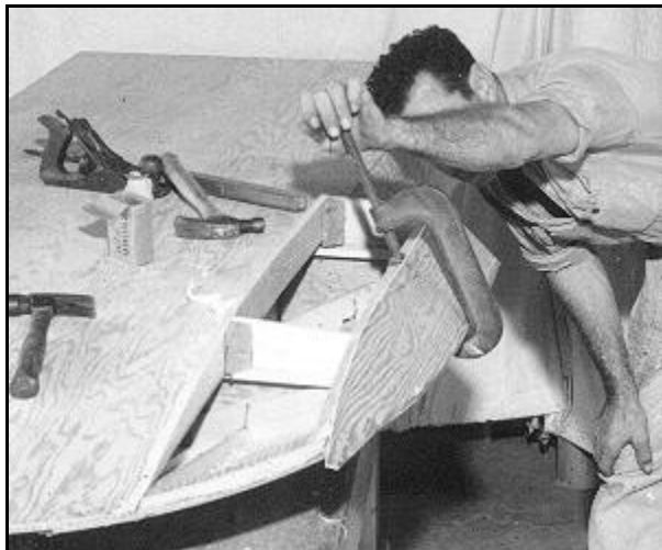
Fig. 13: The hull is turned bottom-side up and the areas for the non-trip and runner planking faired or beveled.
