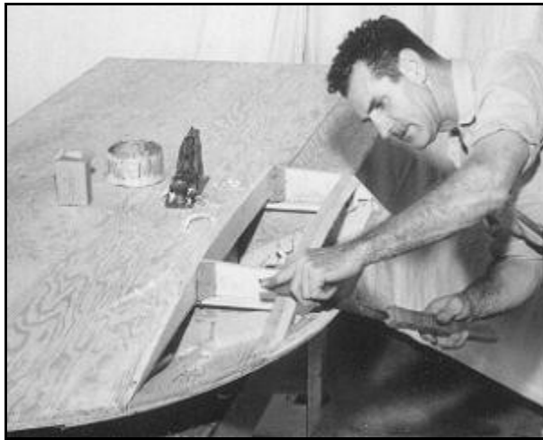
Fig. 13: The hull is turned bottom-side up and the areas for the non-trip and runner planking faired or beveled.
