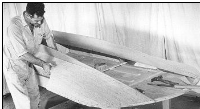
Fig. 11: The coaming is fitted against the carling, notching around the bow piece at the forward portion and around the transom aft.
