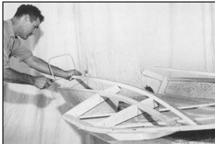
Fig. 6: After mounting the bow piece on the bottom planking, the sheer and carling are tapered to rest on top of the bow piece, fit into the notches in the frames, and extend to the transom for trimming to length.
