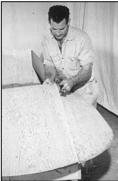
Fig. 17: The cowl plywood is fitted in one side of the coaming rabbet and tacked in place while the other side is fitted.
