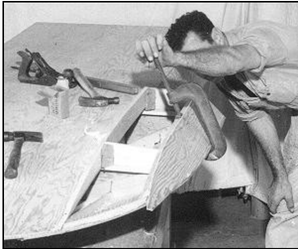
Fig. 14: The non-trip planking is first fastened along the bow piece. Pressure by hand or a clamp is used to spring the non-trip chine so that, as viewed from the side, it is parallel to the runner chine in the aft 9". Fastenings are then driven along the runner chine.
