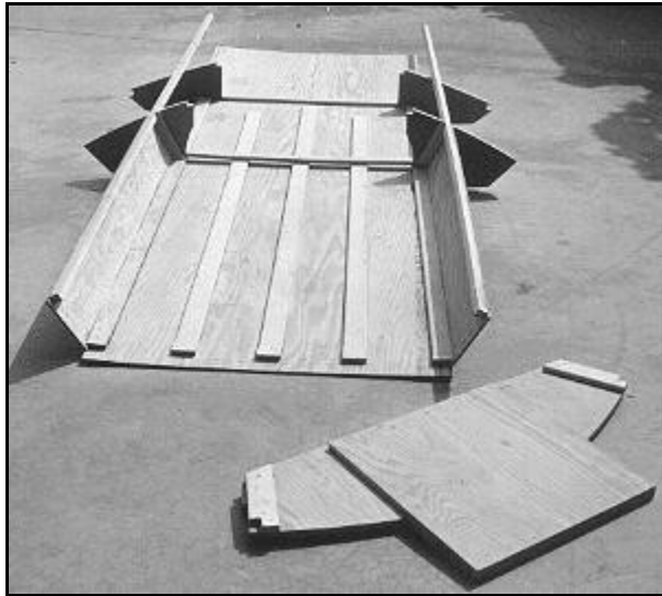
Fig. 3: The side planking sub-assemblies is now installed on the bottom sub-assembly. The transom shown in the foreground is mounted so that the inside surface butts to the battens, chine and sheer and is lapped by the bottom and side planking.
