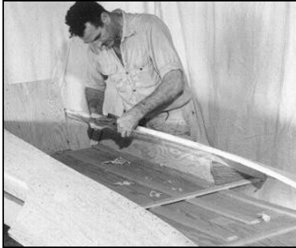
Fig. 10: Fitting of the decking need not be closely done as it can be trimmed after fastening in place. The area along the carling that will mate to the coaming should be carefully trimmed to provide a vertical surface for attaching the coaming.
