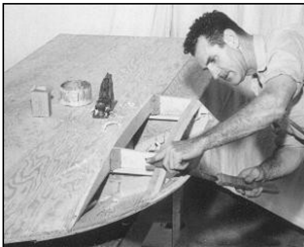
Fig. 13: The hull is turned bottom-side up and the areas for the non-trip and runner planking faired or beveled.
