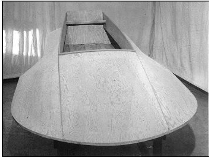
Fig. 18: The completed trimmed hull is ready for paint or fiberglassing. The transom knee is installed 5 1/2" from the top edge of the transom, or closer, depending on the outboard motor used. The cap strip at the dash projects about 3/4" above the decking and covers the exposed edge of the forward decking.
